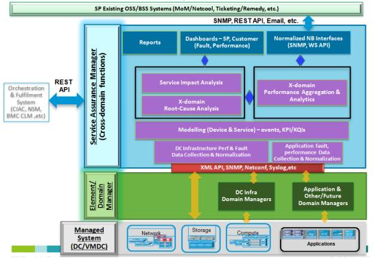
The **Managed Device Layer** consists of Data Center (DC) infrastructure including compute, storage, and network components with instrumentation for inventory, fault, and performance data collection. The instrumentation used in this system includes Simple Network Management Protocol (SNMP), syslog, XML Application Programming Interface (API), NETCONF, vSphere API, and so on. Details of interfaces used per VMDC component are included in Section 3.4 Monitored Components and Services.
