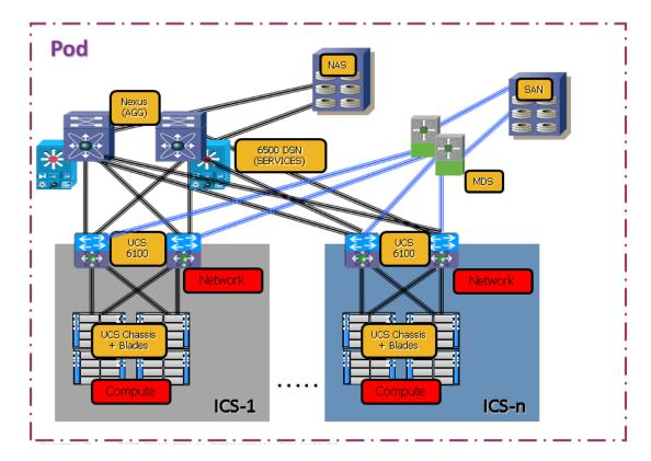
Figure 2-3. VMDC ICS for Scaling the Data Center
