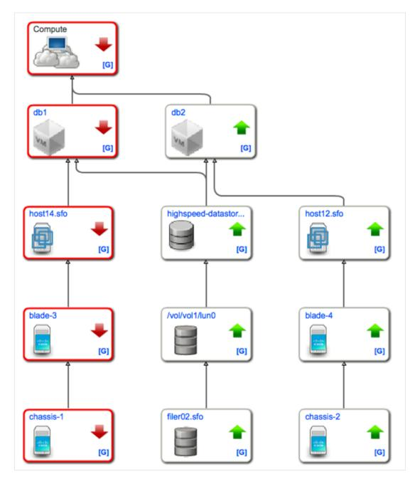
Figure 6-79. Service Impact Graph After Chassis Failure
