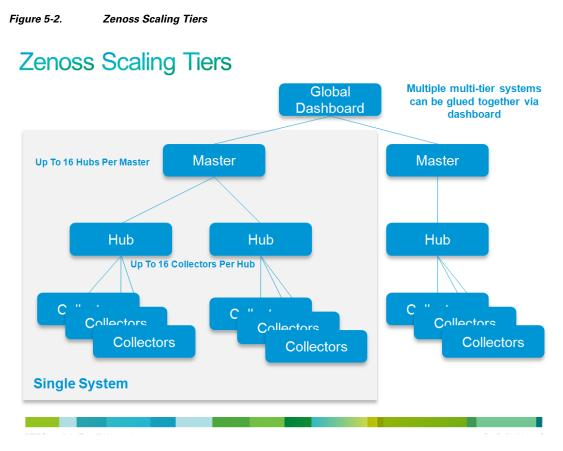
Zenoss CSA recommends sizing increments for lab, Compact Pod, and Large Pod installations, in either a SP IaaS environment or an Enterprise Private Cloud environment. The sizing increments are proportional to the number of large VMDC PoDs deployed to align Zenoss CSA deployment with the VMDC growth model.
