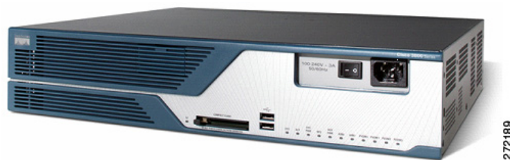
Figure 8 Cisco 3825 Integrated Services Router
