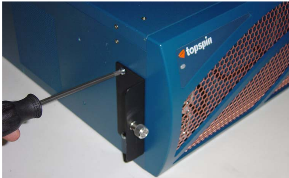
Figure 1-2: Fastening the Side Flanges
