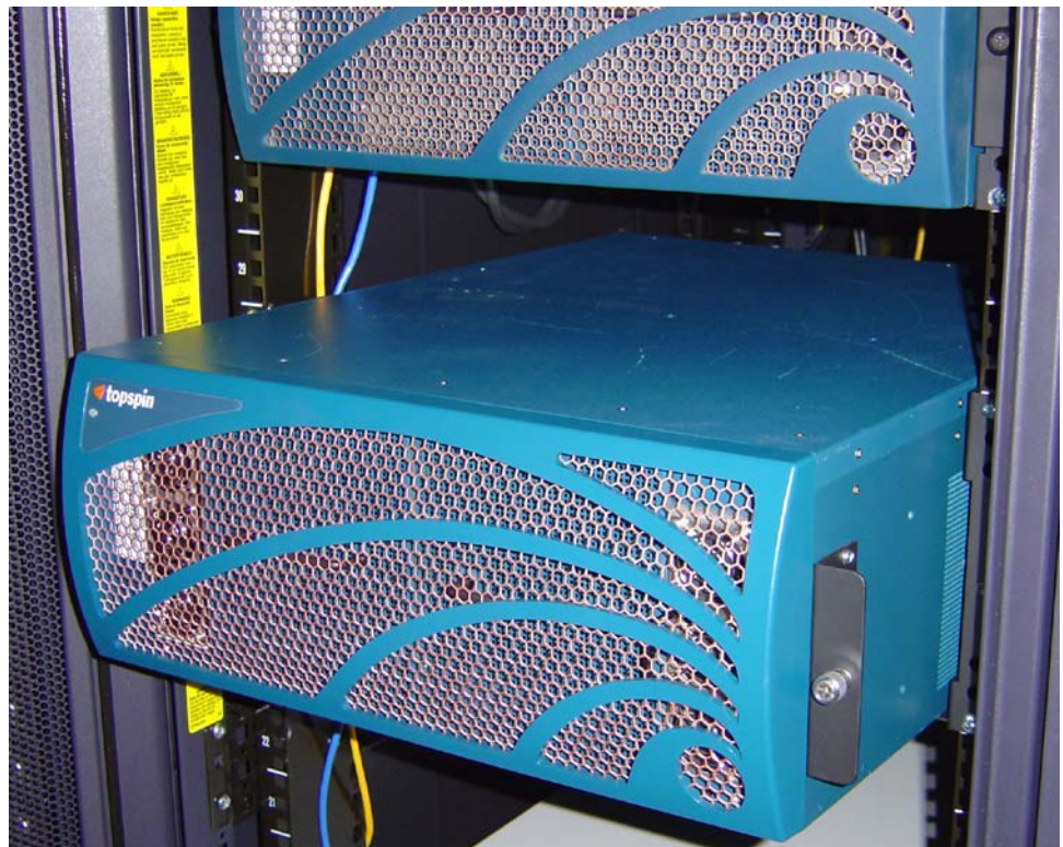
Figure 1-7: Sliding the Chassis onto the Rails
