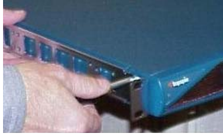
Figure 2-8: Fasten Bracket to Switch Chassis
