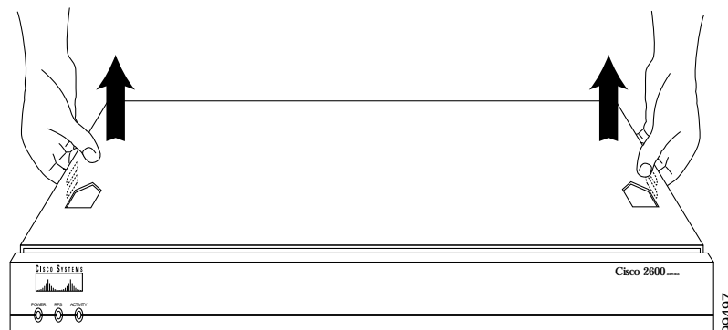
Figure 5 Cisco 2621XM and Cisco 2651XM Chassis Removal
