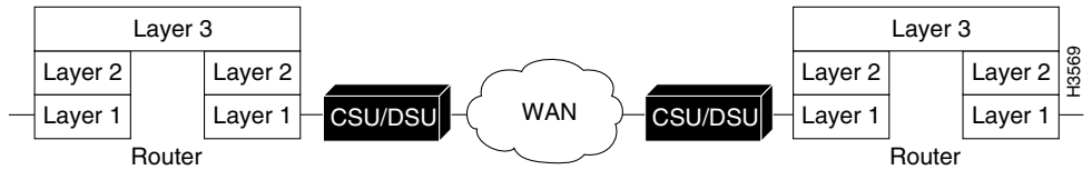
Figure A-4 A Typical WAN Architecture
