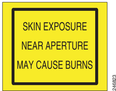
Figure G-13 Burn Hazard Label
