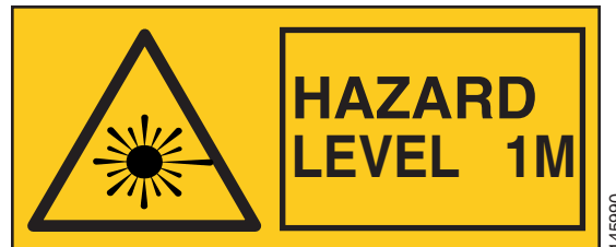
Figure 4-2 Hazard Level Label
