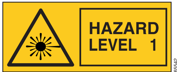
Figure 5-2 Hazard Level Label
