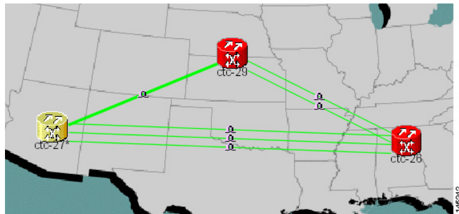
Figure 21-15 Network View with Local Link Consolidation
