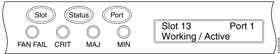
Figure 20-4 Port Status on the LCD Panel
