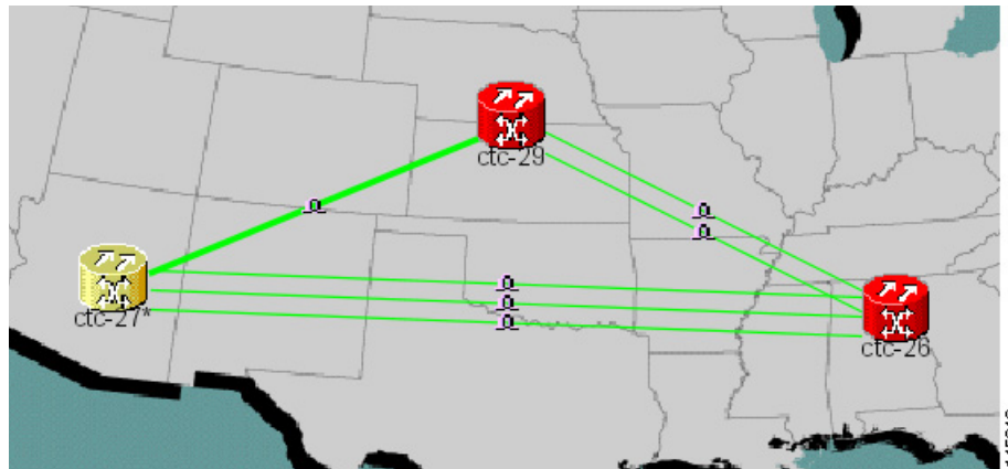
Figure 10-4 Network View with Local Link Consolidation
