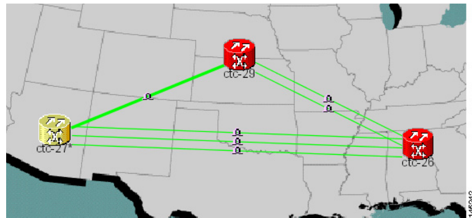
Figure 10-4 Network View with Local Link Consolidation
