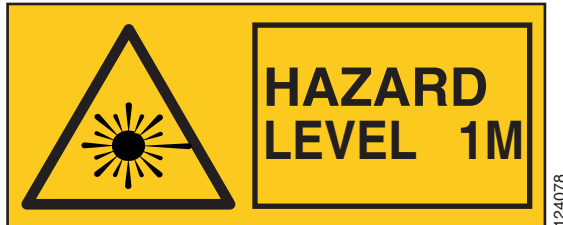
Figure 15-68 Laser Radiation Warning—Hazard Level Label
