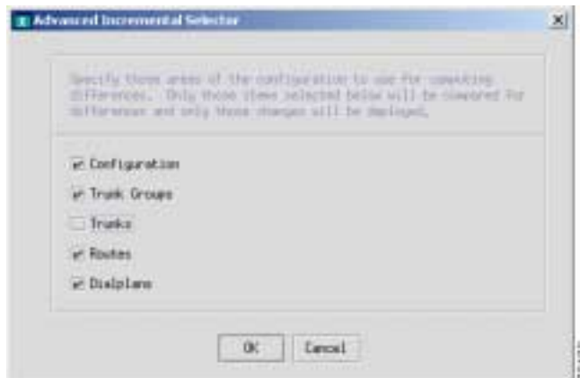
Figure 3-7 Incremental Deployment Component Selector
