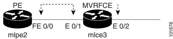
Figure 8-2 MVRFCE PE-CE Link with No CE
