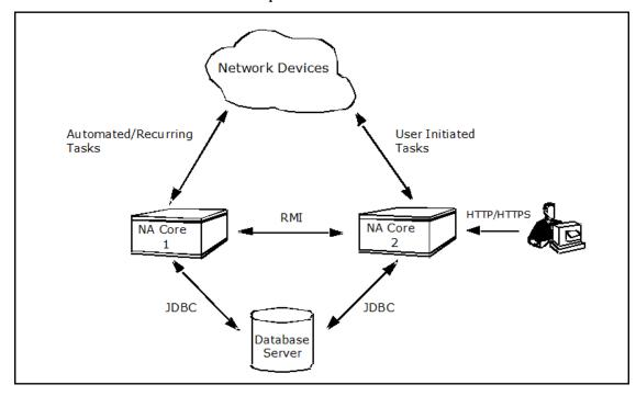
**Topology 4:** Using one server for all user-interaction, while another server is used for all device tasks. This is useful if NCM users experience UI performance limitations due to device tasks loads on a specific NCM Core. You should use this topology if users run multiple search and reporting operations that impact overall system performance.
