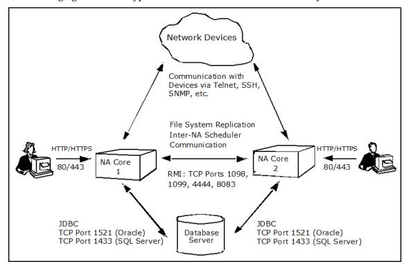
The following figure shows a typical two-NCM Core Horizontal Scalability installation.
