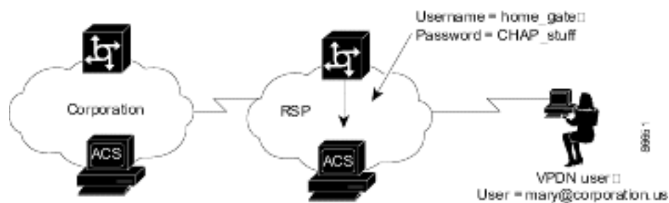
Figure D-7 NAS Authenticates Tunnel with ACS
