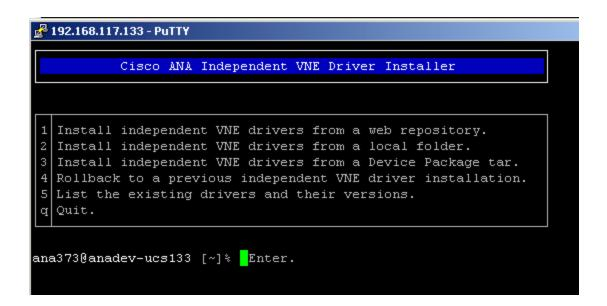
5. Choose option **4** (*Rollback to a previous independent VNE driver installation*) and press Enter at the prompt. The installation script creates a log and prompts you for the full pathname of the folder that contains the backup file with the desired rollback configuration.
