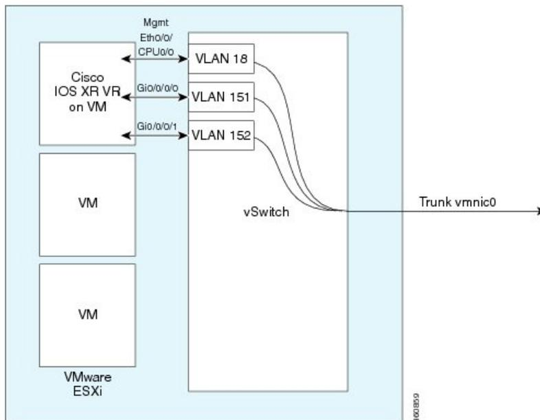
The figure below shows an interface of a Cisco IOS XRv Router being mapped directly to a trunk interface on the vSwitch trunk.
