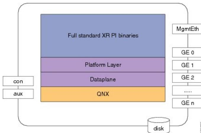
The Cisco IOS XRv Router platform image (figure above) is made up of these major components:
