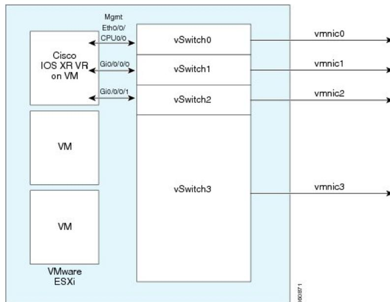
This figure shows multiple Cisco IOS XRv Router interfaces sharing one host VMware ESXi Ethernet interface.
