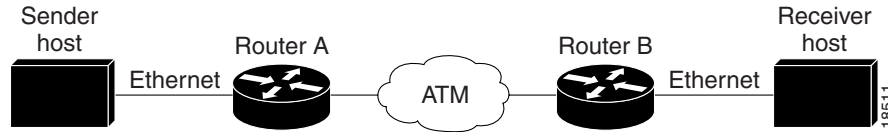
Figure 24 Example RSVP-ATM QoS Interworking Configuration
