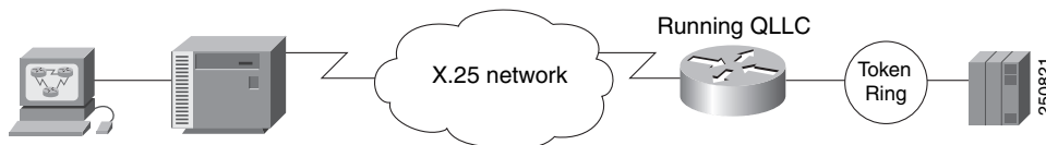
Figure 4 Router Running QLLC Conversion Feature
