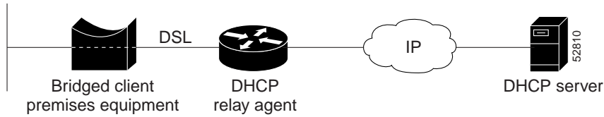
Figure 1 Network Topology Using ATM RBE and DHCP
