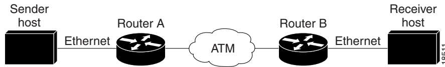
Figure 14 Example RSVP-ATM QoS Interworking Configuration
