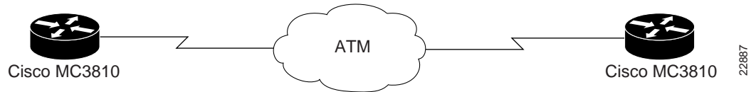
Figure 93 Sample Configuration: Two Cisco MC3810s Using ATM SVCs for Voice
