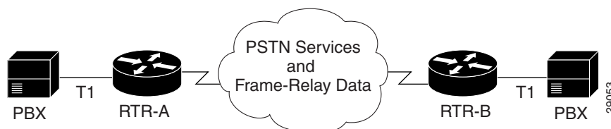
Figure 3 Sample Configuration: Drop and Insert with Data and PSTN Voice Services
