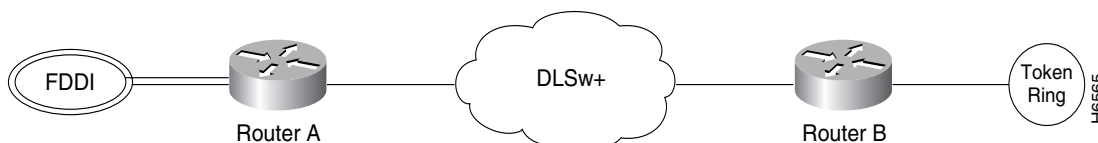
Figure 89 DLSw+ Translation between FDDI and Token Ring
