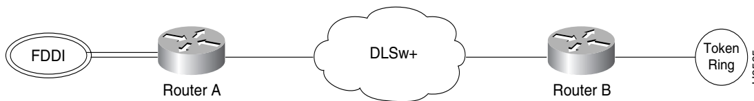
Figure 86 DLSw+ Translation between FDDI and Token Ring
