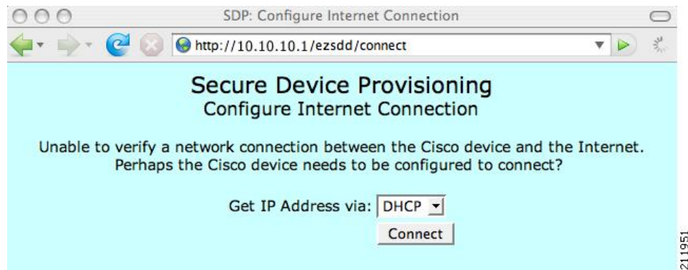
Figure 7 Sample Connect Page for DHCP IP Address Assignment Method
