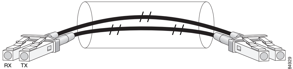
Figure 3-26 LC-Type Cable for the XFP Optical Transceiver Modules
