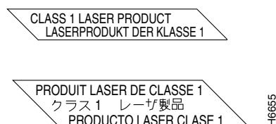
Figure 4-1 Class 1 Laser Warning Labels for Single-Mode Port
