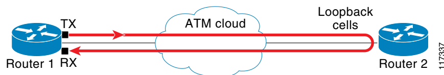
Figure 8-3 Performing a Local Loopback—Router Level
