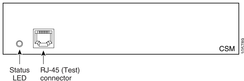
Figure 1-1 Content Switching Module Front Panel
