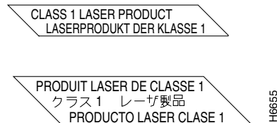
Figure 2-1 Class 1 Laser Warning Labels on DPT Port Adapter for Single-Mode Port
