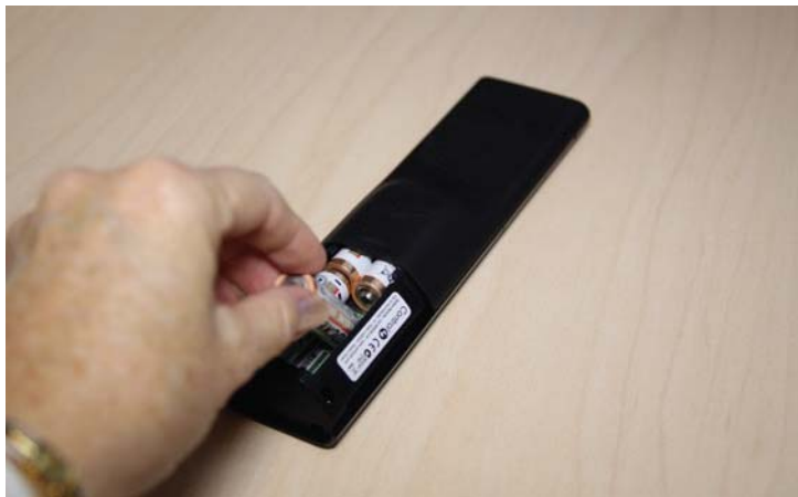
Figure 4 Remove the Old Batteries
