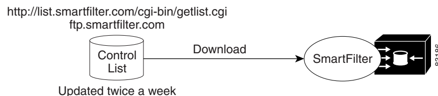
Figure 1-5 Subscription to the Control List Allows Access to the Latest URL Database
