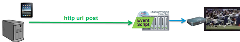
Figure 3 Input Sources of Contact Closure to Cisco StadiumVision Director
