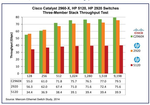
Stacking throughput of the C2960-X stack exceeded that of the HP 2920 and HP 5120 for frame sizes ranging from 512 to 9198 bytes. The greatest throughput achieved by the C2960-X stack was 99.58% (79.5 Gbps out of the theoretical maximum throughput of 80 Gbps) for9198-byte frames. Minimum frame size of 100 bytes was needed as we also verified data integrity and correct sequencing. Longer bars depict better performance.
