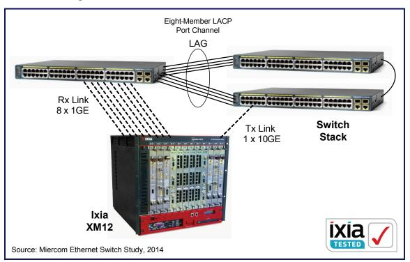
Four 1GE ports on each switch in the two member stack were configured in a port channel, forming an eight-member LACP group to send traffic. Also, eight 1GE ports on each standalone switch (lower left) served as a LACP group to receive traffic.
