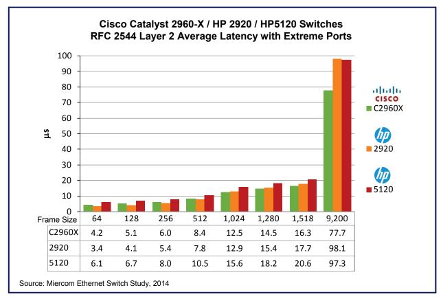
Based on RFC 2544, Layer 2 latency for the Cisco Catalyst 2960-X and the HP 2920 and 5120E switches is shown as an average calculated from small to jumbo frame sizes ranging from 64- to 9200-bytes (jumbo). The C2960-X switch had over 20% lower average latency for the jumbo frame size when compared to the HP 2920 and HP 5120. Shorter bars depict better performance.
