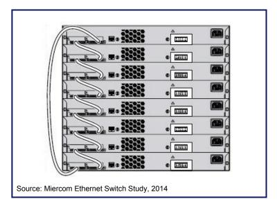
A FlexStack-Plus module has been installed in each Catalyst 2960-X Series switch in this drawing of an eight-member stack. The modules, on the left, are connected by Cisco cabling.
