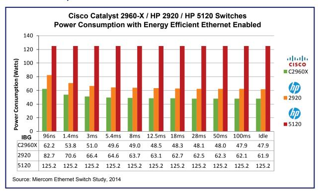
Testing verified that power savings with EEE enabled increased for both Cisco C2960-X and HP 2920 switches with EEE enabled as the IBG increased. The C2960-X utilized just under one-quarter less power than the HP 2920 for each IBG. HP 5120 does not support EEE and power consumption will be same as with full Traffic load. Shorter bars depict better performance.
