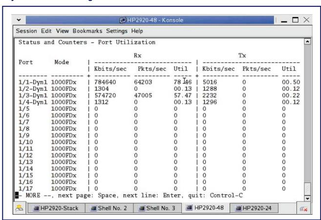
The HP 2920 failed to perform perfect load balancing after the 1GE link was removed. As a result, traffic was lost.
