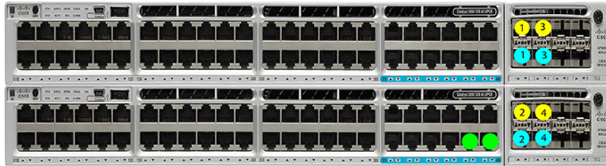
Dual 10/25GE ToR Switches (standalone or stacked)
