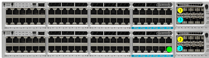
Dual 10/25GE ToR Switches (standalone or stacked)
