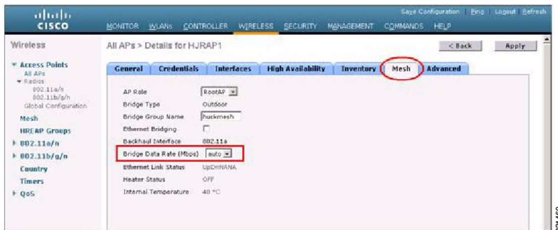
Figure 12: Bridge Rate Set to Auto
