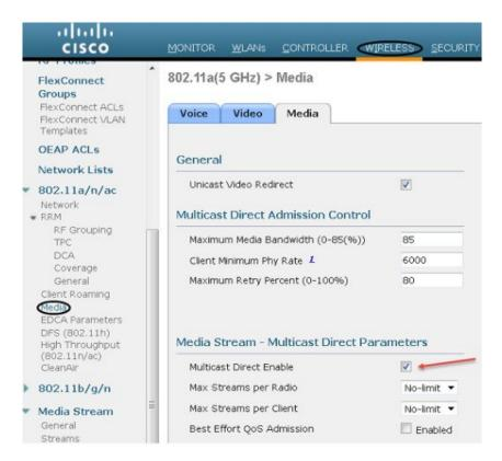
The Unicast Video Redirect is enabled by default. This will allow unicast video traffic flow to wireless clients.
