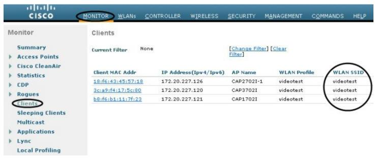
The associated clients have an IP address and good uplink connectivity to the access point.
