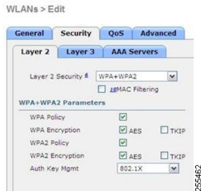
Figure 7: Compatible Security Settings for OEAP Series
