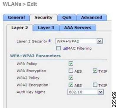
Figure 5: Incompatible WPA and WPA2 Security Encryption Settings for OEAP 600 Series
