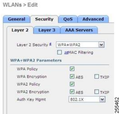
Figure 7: Compatible Security Settings for OEAP Series
