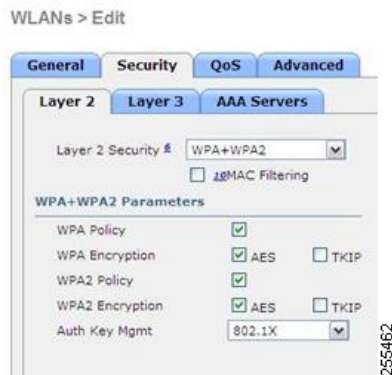
Figure 7: Compatible Security Settings for OEAP Series
