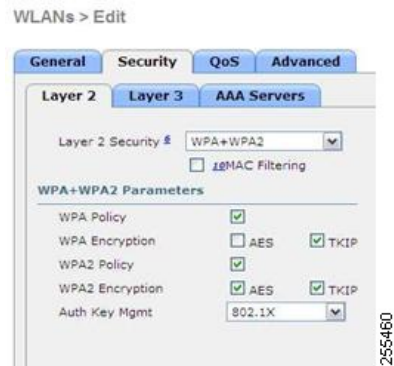
Figure 5: Incompatible WPA and WPA2 Security Encryption Settings for OEAP 600 Series
