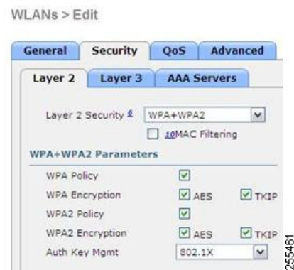
Figure 6: Compatible Security Settings for OEAP Series
