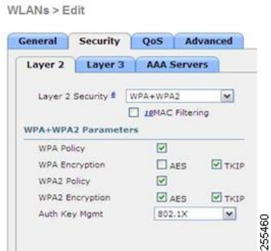
Figure 5: Incompatible WPA and WPA2 Security Encryption Settings for OEAP 600 Series
