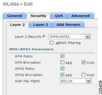
Figure 7: Incompatible WPA and WPA2 Security Encryption Settings for OEAP 600 Series
