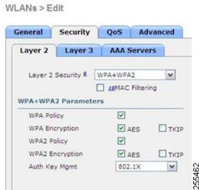
Figure 9: Compatible Security Settings for OEAP Series
