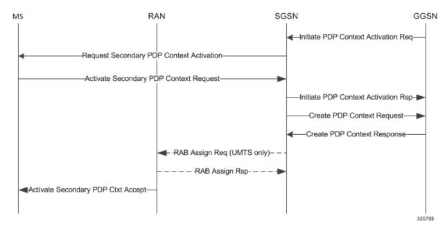
Figure 66: Call Flow: Successful Network Requested Secondary Activation (Gn/Gp)
