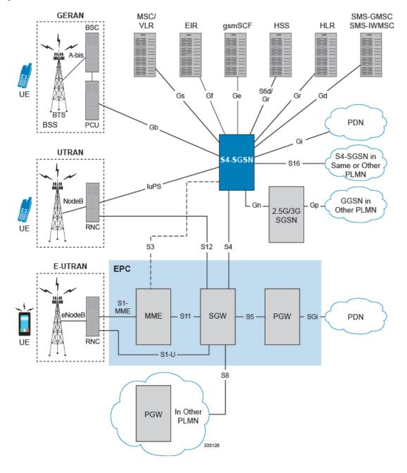
Figure 3: S4-SGSN Network Architecture
