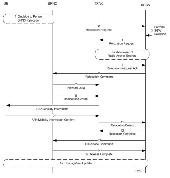
Figure 104: Intra-S4-SGSN SRNS Relocation without SGW Relocation
