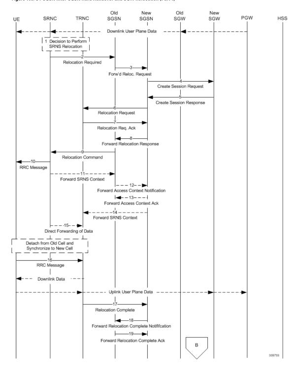
Figure 108: S4-SGSN Inter-SGSN Hard Handover and SGW Relocation (Part 1)
