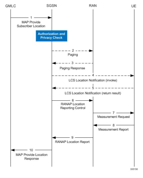
Figure 55: 3G Mobile Terminating Location Request
