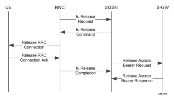
Figure 34: Iu Release Procedure with Direct Tunnel
