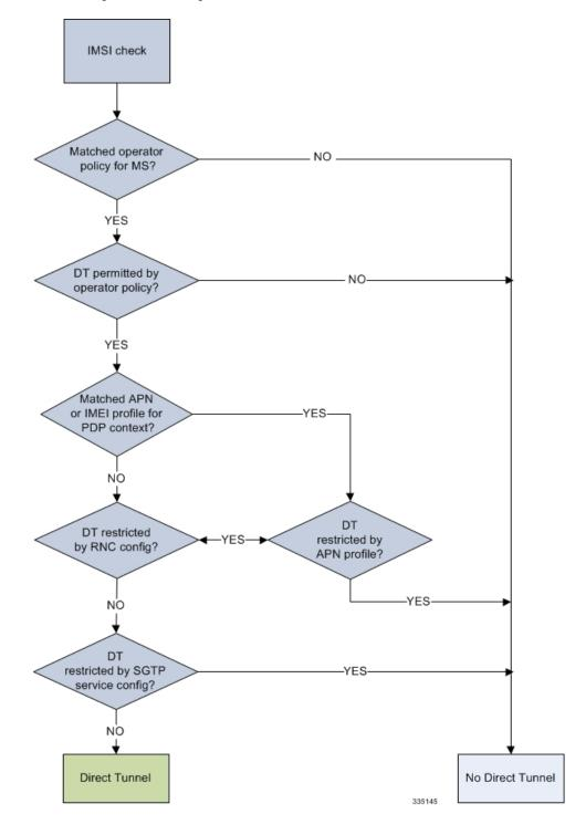
Figure 30: Direct Tunneling - Establishment Logic
