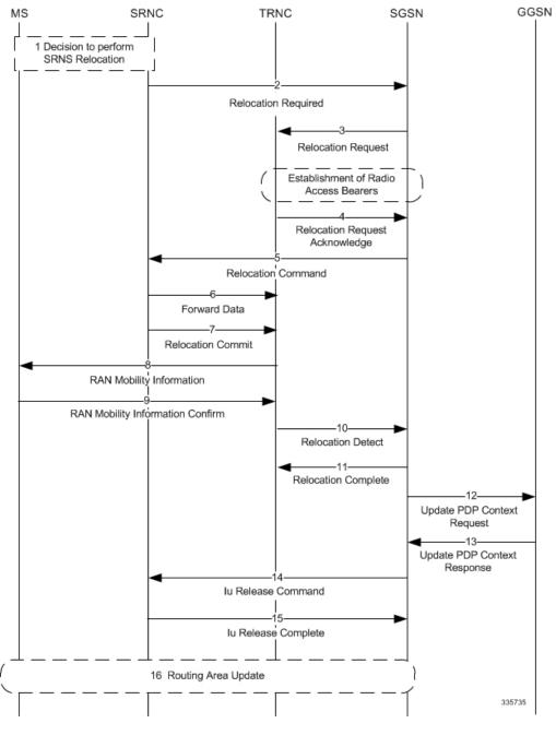
Figure 100: Intra-SGSN Gn/Gp SRNS Relocation Call Flow
