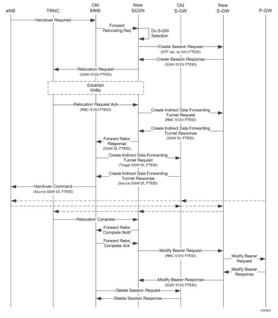
Figure 43: New SRNS with S-GW Change and Indirect Data Transfer
