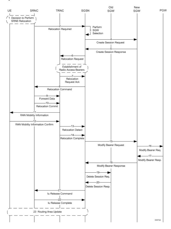
Figure 105: Intra-S4-SGSN Relocation with SGW Relocation
