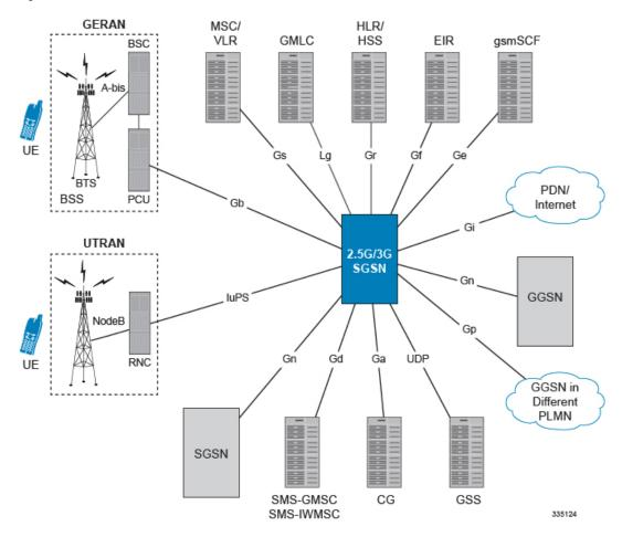
Figure 1: 2.5G and 3G Dual Access Architecture
