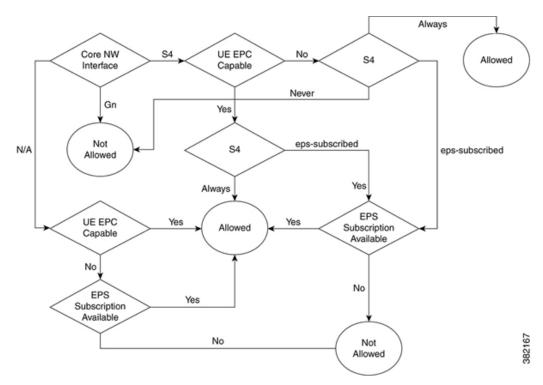
When the S4 interface is allowed, APN selection is performed based on the following logic:
