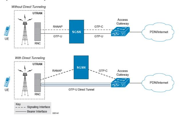
A direct tunnel improves the user experience (for example, expedites web page delivery, reduces round trip delay for conversational services) by eliminating switching latency from the user plane. An additional advantage, direct tunnel functionality implements optimization to improve the usage of user plane resources (and hardware) by removing the requirement from the S4-SGSN/S-GW to handle the user plane processing.
