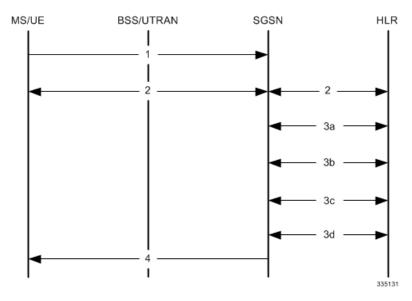
This simple attach procedure can connect an MS via a BSS through the Gb interface (2.5G setup) or it can connect a UE via a UTRAN through the Iu interface in a 3G network with the following process:
