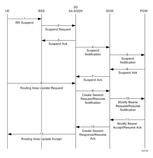
Figure 85: Intra-SGSN Suspend Procedure with Intra-RAU as Subsequent Procedure
