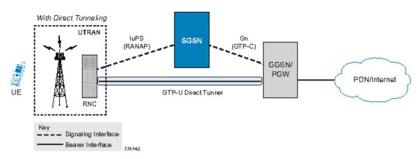
• Gn/Gp Interface towards P-GW When Gn/Gp interworking with pre-release 8 (3GPP) SGSNs is enabled, the GGSN service on the P-GW supports direct tunnel functionality. The SGSN establishes a user plane (GTP-U) tunnel directly between the RNC and the collocated PGW, using an Update PDP Context Message toward the GGSN/P-GW.
