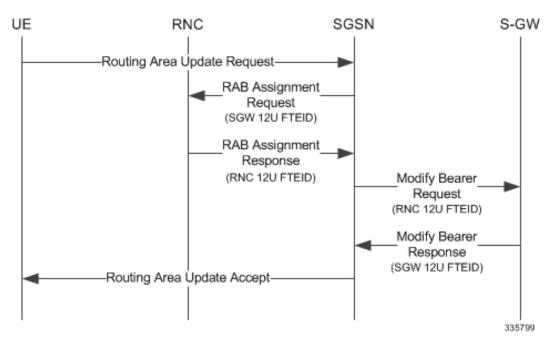
Figure 38: Routing Area Update Procedure without SGW Change
