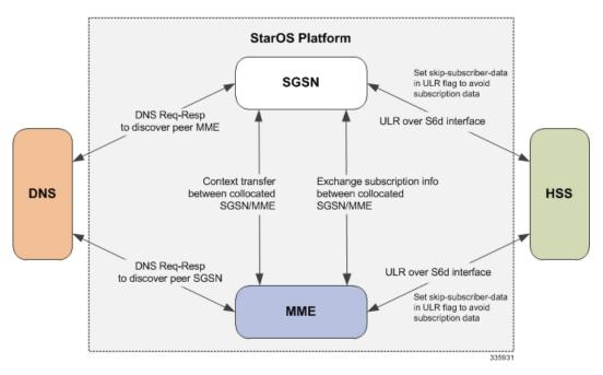
The above diagram displays the interworking of various modules when the Combo Optimization feature is enabled in a co-located SGSN-MME setup.
