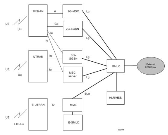
The SGSN informs the HLR/HSS regarding the LCS capabilities of UE in GPRS (2G) or UMTS (3G) networks. The SGSN may include the IP address of the V-GMLC associated with the SGSN in the MAP\_UPDATE\_GPRS\_LOCATION message during Attach and ISRAU procedures.
