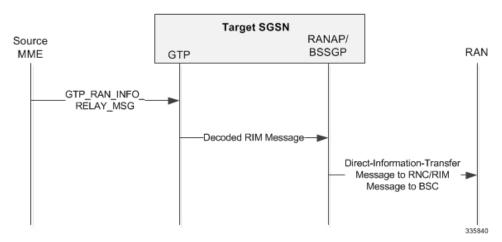
In this case, the SGSN has to decode the incoming GTP message correctly and forward the RIM message to the destination RNC/BSS.
