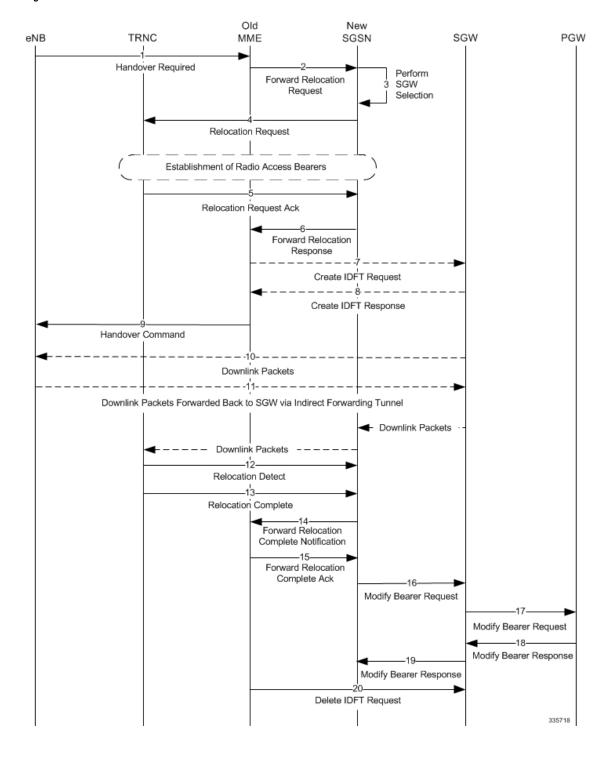
Figure 106: S4-SGSN E-UTRAN to UTRAN Connected Mode Handover without SGW Relocation Call Flow
