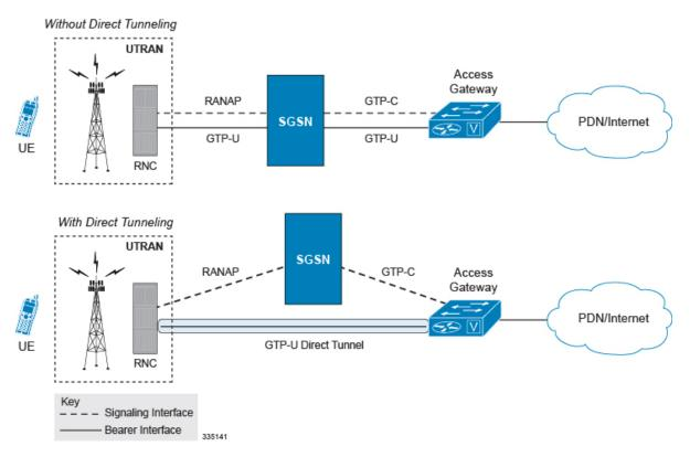
A direct tunnel improves the user experience (for example, expedites web page delivery, reduces round trip delay for conversational services) by eliminating switching latency from the user plane. An additional advantage, direct tunnel functionality implements optimization to improve the usage of user plane resources (and hardware) by removing the requirement from the SGSN to handle the user plane processing.
