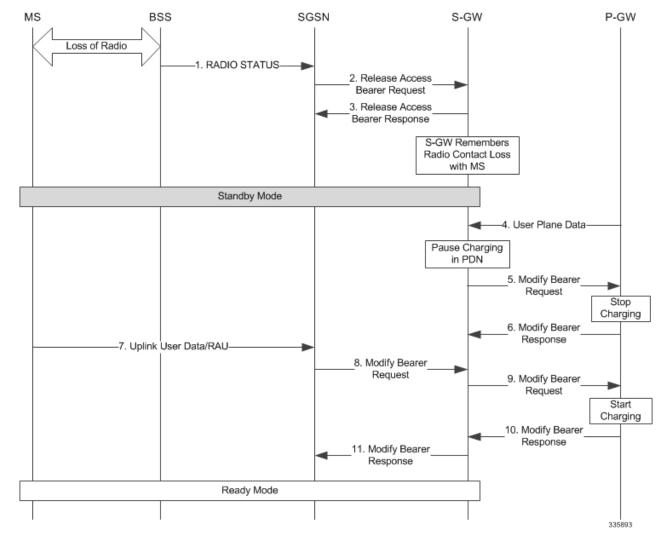
Figure 57: 2G Ready-to-Standby State Transition Using S4
