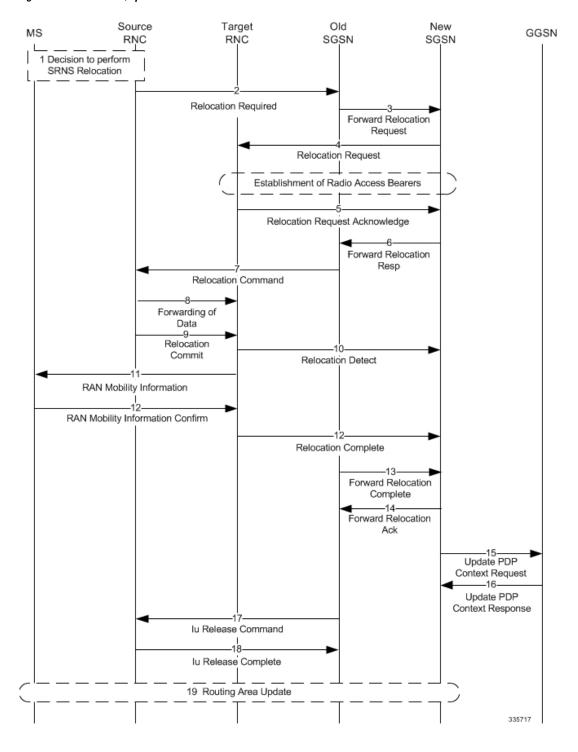
Figure 99: Inter-SGSN Gn/Gp SRNS Relocation Call Flow
