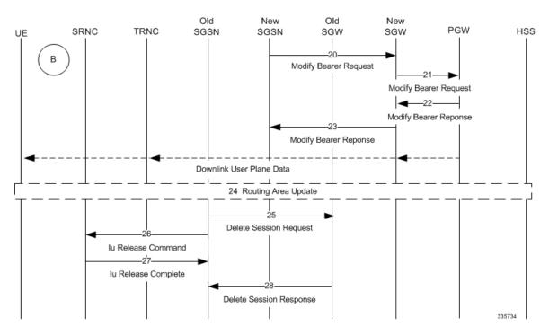
Figure 109: S4-SGSN Inter-SGSN Relocation with Hard Handover and SGW Relocation (Part 2)
