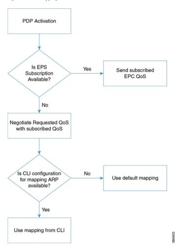
Figure 75: QoS Mapping from SGSN to SGW/PGW
