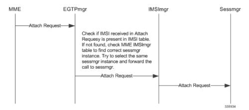
Listed below is the SessMgr instance selection logic during an Attach procedure:
