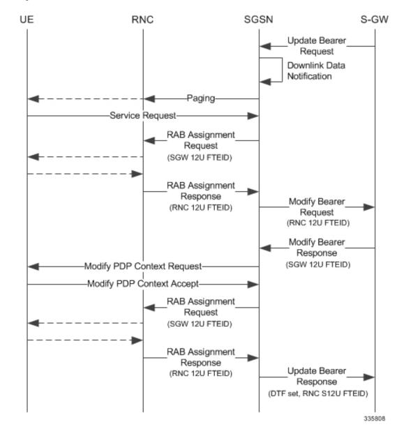
Figure 47: PGW Init Modification when UE in Idle State
