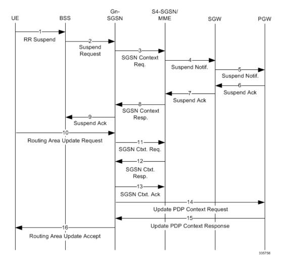
Figure 86: Inter-SGSN Suspend and Resume Procedure with Peer S4-SGSN/MME
