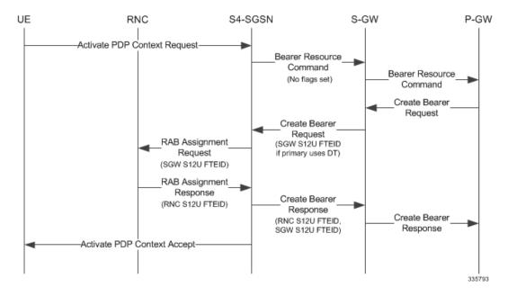
Figure 32: Secondary PDP Activation with Direct Tunnel
