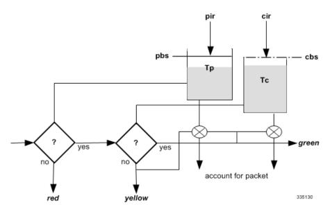
The policing function compares the data unit traffic with the related QoS attributes. Data units not matching the relevant attributes will be dropped or marked as not matching, for preferential dropping in case of congestion.
