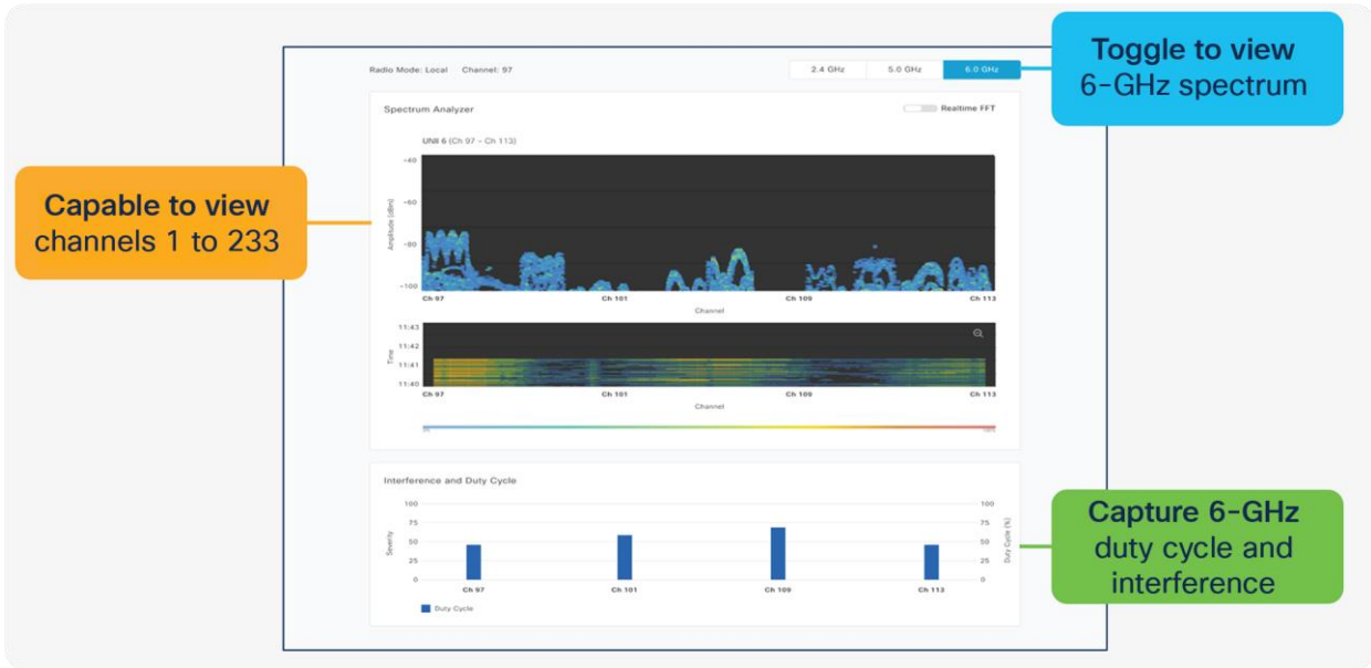
Figure 45. Spectrum analysis - Visualize RF spectrum energy, not only for 2.4 and 5 GHz, but now also for 6 GHz
