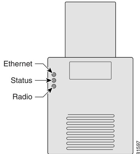
The LEDs signals have the following meanings (for additional details refer to [Table 5-1](#)):
