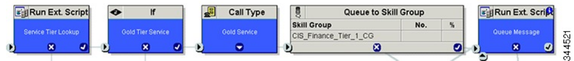
Figure 1: Changing a Call Type Prior to the Queue to Skill Group Node
