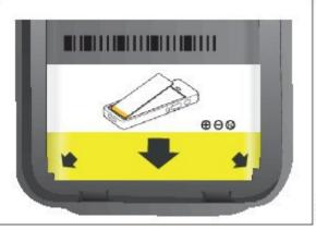
a) Hold the battery so that the lower edge is close to the bottom of the compartment. Make sure that the metal contacts on the phone and battery face each other. On the battery, the Cisco logo must be near the locking catch and the arrow must point to the base of the phone.
