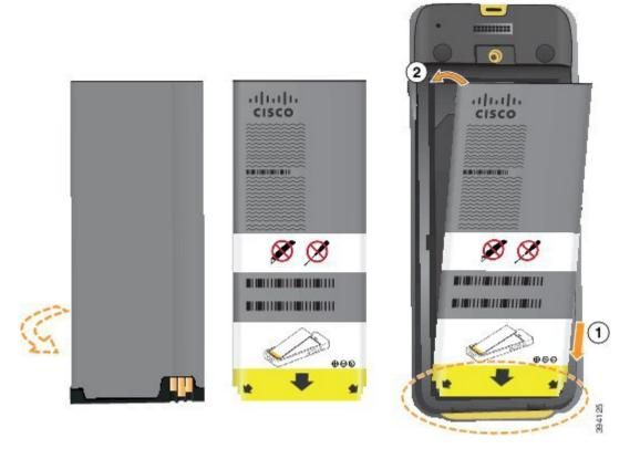
The battery has metal contacts that must connect to the contacts in the battery compartment. The battery also has an arrow at the bottom and the Cisco logo at the top.
