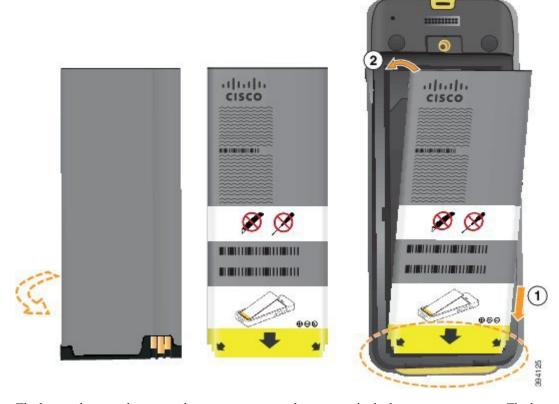
The battery has metal contacts that must connect to the contacts in the battery compartment. The battery also has an arrow at the bottom and the Cisco logo at the top.
